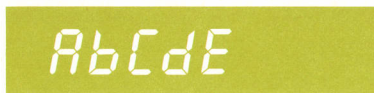
Fig. 4. The seven-segment font used in the HP-15C's liquid-crystal display allows representations of the alphabetic characters A, B, C, D, and E as shown above for use in labeling matrices.
